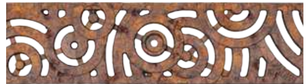
Design grating, CELTIQ, cast iron, uncoated Load classes: C250, Length: 50 cm, SW 10 mm
