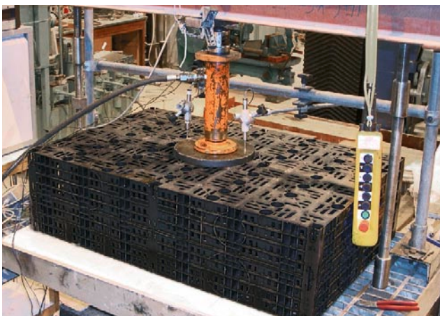
Test with point load from above
