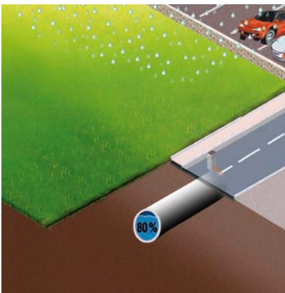
Figure 1: Original condition of site. Rainwater can soak away into the open soil. Utilisation of drains max. 80 %.
