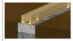
Position channel string, sump unit and end cap on the concrete bed.
